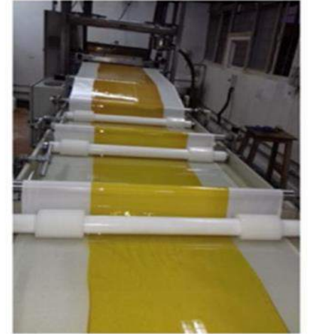
Continuous casting of PA-doped PBI Membrane
