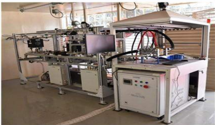
Demonstration of 3 kW e LT-PEMFC System for telecom tower applications (Industry Partner: RIL)
