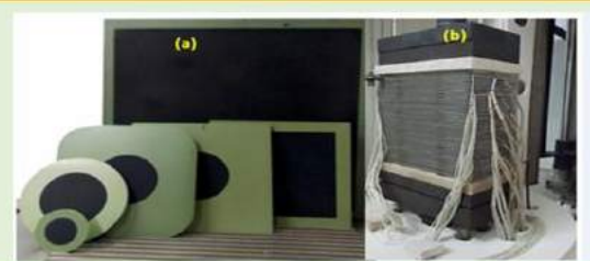
SOFC for High Temp. Steam Electrolyser
