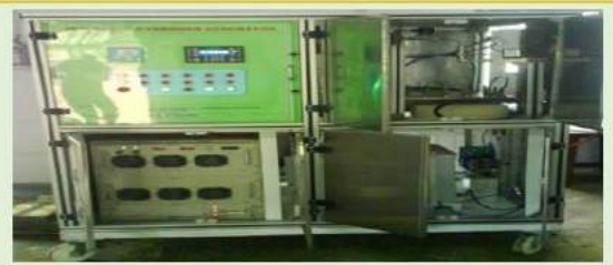
PEM Water Electrolyser Unit (1 Nm 3 /h)
