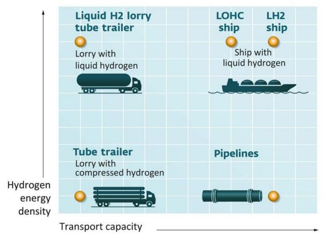
Liquid organic hydrogen carriers (LOHC): Organic compounds that can absorb and release hydrogen through chemical reactions say Toluene / methylcyclohexane
