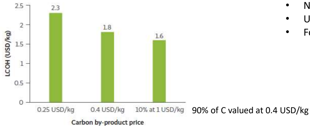
Figure 11 Utilising thermo-catalytic pyrolysis could allow for a much higher value of carbon by-product
