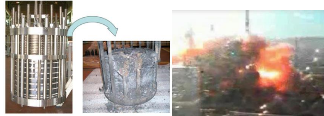
Titanium electrolyser before and after the accident
