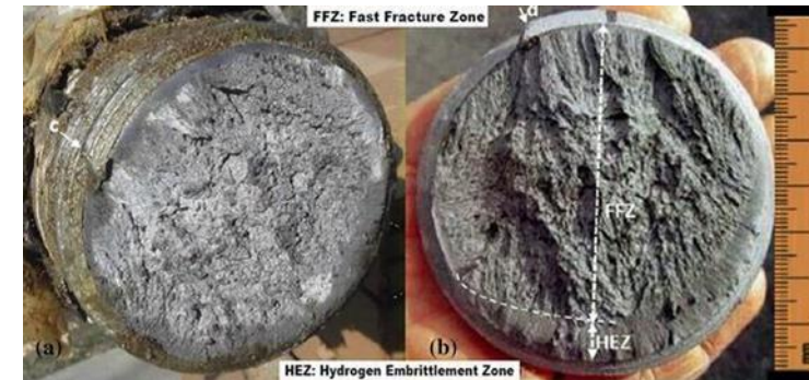
Fracture face of Hot dip galvanized high strength steel anchor rods
