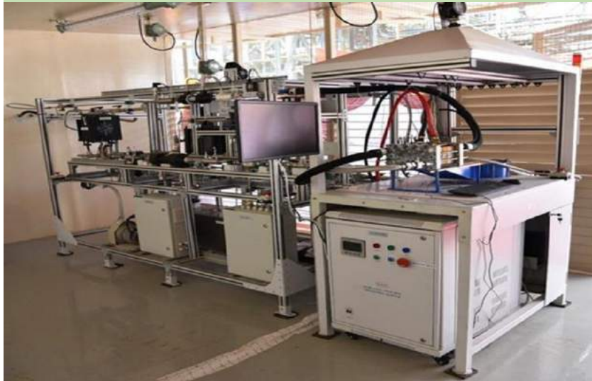
Demonstration of 3 kWe LT-PEMFC System for telecom tower applications
