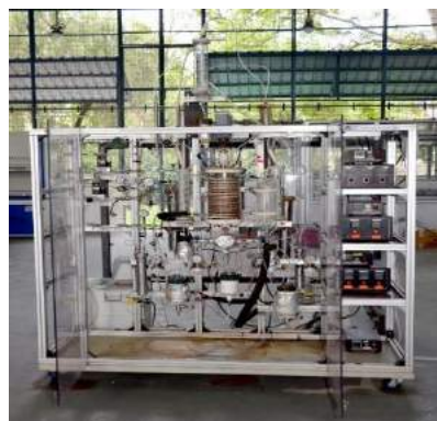
Bunsen reaction set-up
